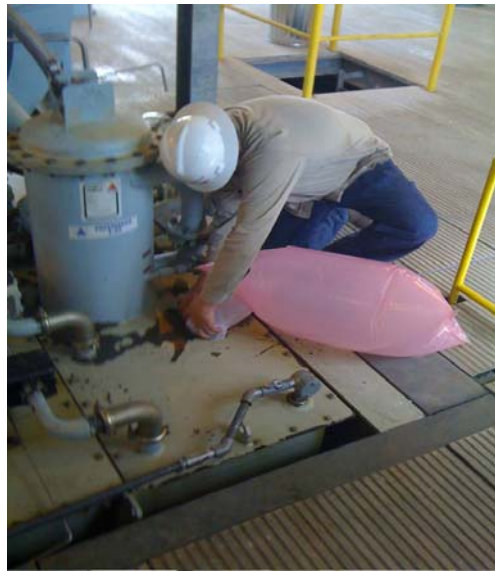
Figure 2-9. Centrifugal Compressor Seal Oil Gas Measurement Using Calibrated Bag Technique
