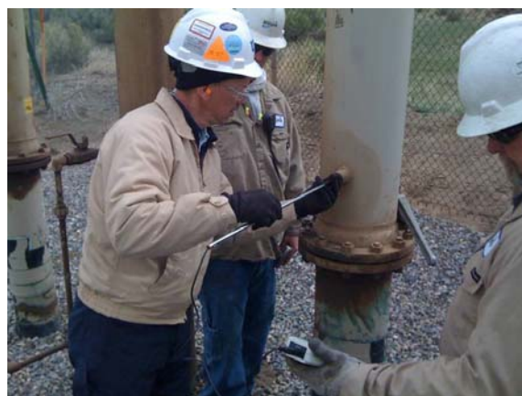
Figure 2-5. Sampling a Blowdown Vent with Hot Wire Anemometer
