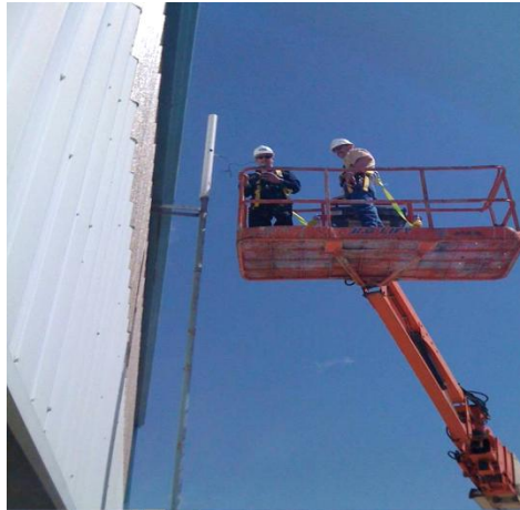
Figure 2-7. Sampling a Rod Packing Vent Stack with Enclosed Rotary Vane Anemometer
